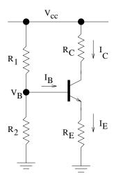
Figure 20: Basic transistor current source.
