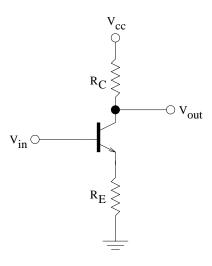
Figure 21: Basic common-emitter amplifier.
