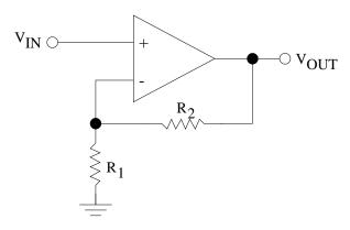
Figure 31: Non-inverting amplifier configuration.
