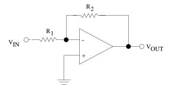
Figure 30: Inverting amplifier configuration.
