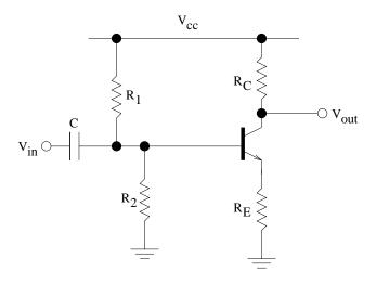
Figure 22: Common-emitter amplifier with input network.
