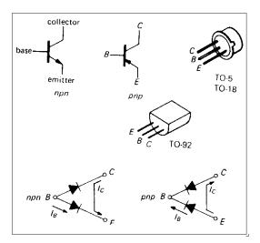
Figure 16: Bipolar transistor connections.
