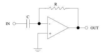
Figure 34: Op-amp differentiator or high-pass filter.
