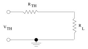
Figure 5: The Thevenin equivalent circuit.
