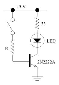
Figure 18: A transistor switch.
