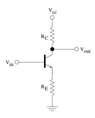
Figure 27: Basic common-emitter amplifier.
