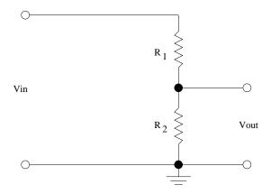
Figure 3: A voltage divider.
