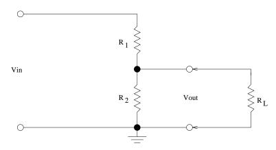
Figure 4: Adding a "load" resistor  $R_L$ .
