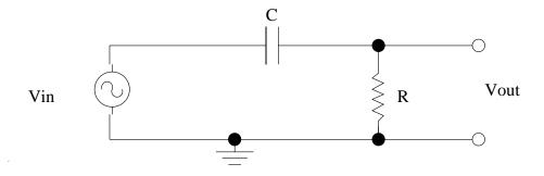
Figure 10: A high-pass filter.
