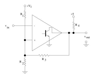
Figure 39: Schmitt trigger.
