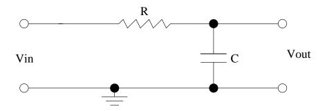
Figure 11: A low-pass filter.
