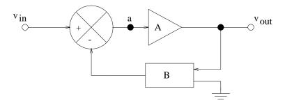
Figure 35: General negative feedback configuration.
