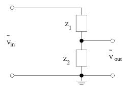
Figure 9: The voltage divider generalized.
