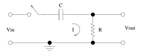
Figure 8: RC circuit — differentiator.
