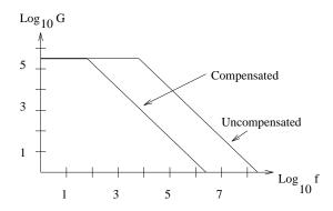
Figure 37: Bode plot showing effect of op-amp compensation.
