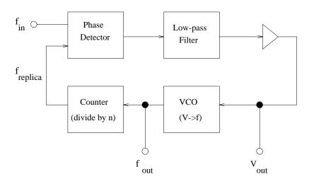
Figure 45: PLL schematic.  $V_{\rm out}$  provides the FM signal.
