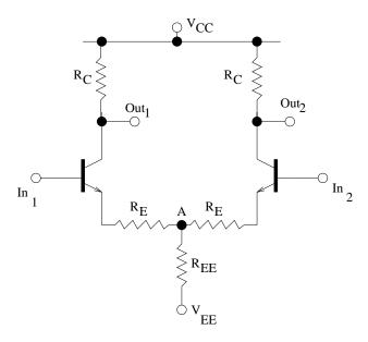
Figure 25: Differential amplifier design.
