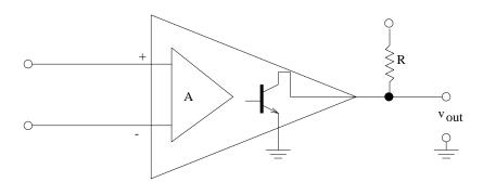
Figure 38: Comparator model.
