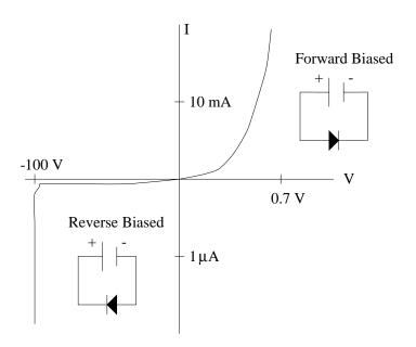
Figure 15: The V-I behavior of a diode.
