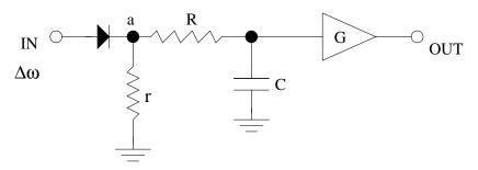
Figure 44: Simple AM receiver.
