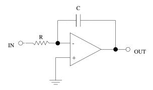
Figure 33: Op-amp integrator or low-pass filter.
