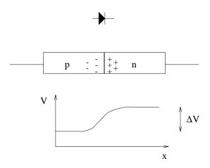
Figure 14: A pn junction, forming a voltage gap across the junction.
