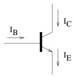
Figure 17: Transistor currents.
