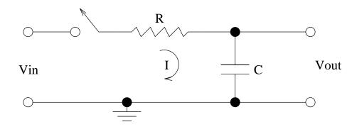
Figure 7: RC circuit — integrator.
