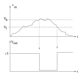
Figure 40: Examples of Schmitt trigger signals versus time. Top:  $v_{\rm in}$ ; the dashed lines indicate the two thresholds set up at the + input of the comparator. Bottom:  $v_{\rm out}$ .
